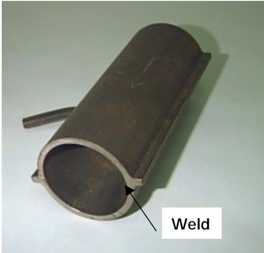
2.5" x .155" steel fin boiler tube
